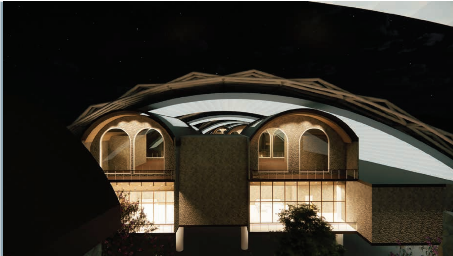
BENEATH THE SECONDARY ARCHWAYS, REFLECTIVE MEMBRANES SIMULATE A BRIGHT DAY SKY DURING THE NIGHT.
