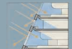
B) AFTER: SLOPED SOUTH FACADE
